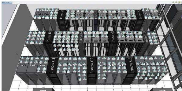
Figure 4. Power consumption or Thermal heat load at the rack location monitoring of the data center
